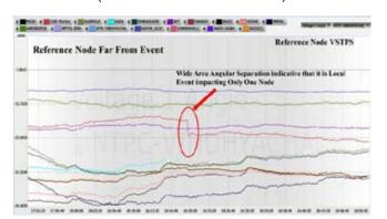
Fig. 8 : Wide area angular separation when the reference node selected far from the event/disturbance location
