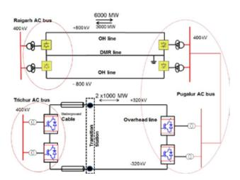
Fig. 2 : Common Pugalur Converter bus for Raigarh-Pugalur LCC and Pugalur -Trichur VSC HVDC Links
