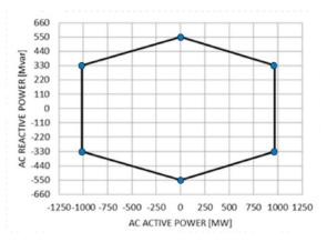
The above capability requirements are valid for AC system voltage between 380-420 kV. If AC voltage is outside this range then restrictions at some point may appear. The capability of converter varies based on following factors- AC system voltage, frequency and DC voltage.
