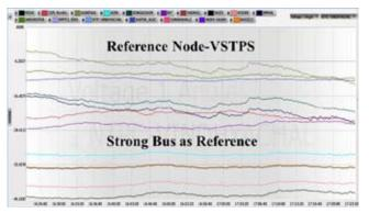
Fig. 4 : Strong Bus/Node in SR grid used as a reference for Wide Area Angular Separation Monitoring
