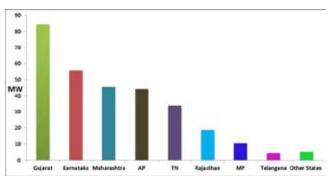
Fig. 3 : Wind potential at 100 m hub height (Source:NIWE)
