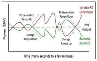
Fig. 5 : Variable RE and Storage Ramping
