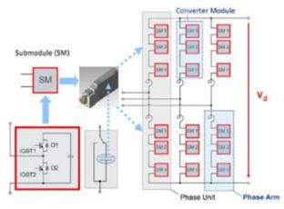
Fig. 4 : Typical VSC-HVDC multi-level topology<sup>[4]</sup>
