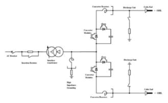
Fig. 3 : Overview Diagram for Converter station (Trichur end) for Pugalur -Trichur VSC HVDC Link
