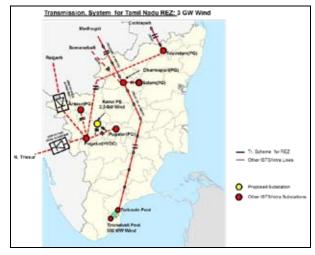
Fig. 9 : Transmission scheme for renewable energy zones in Tamil Nadu (Ph-I : 3 GW)
