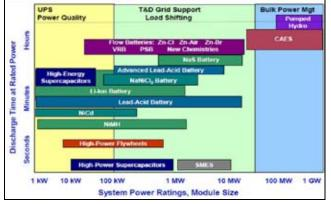
Fig. 2 : Power rating and rated Energy capacity<sup>[05]</sup>
