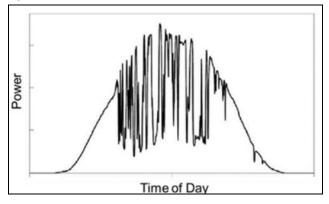
Fig. 4 : Power output from solar during a typical summer day having random cloud cover
