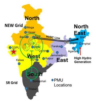
**Fig. 2** : Indian Grid shown as the synchronous interconnection of five regional grids. Nodes with PMU are shown in blue. Node with Event, HVDC Line, Varying High Hydro Generation Complex is highlighted for case studies reference.
