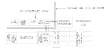
Fig. 2 : Synchronous Condenser Building – Equipment Layout
