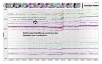
Fig. 11 : Wide area angular separation when the reference node is selected near to the source of LFO
